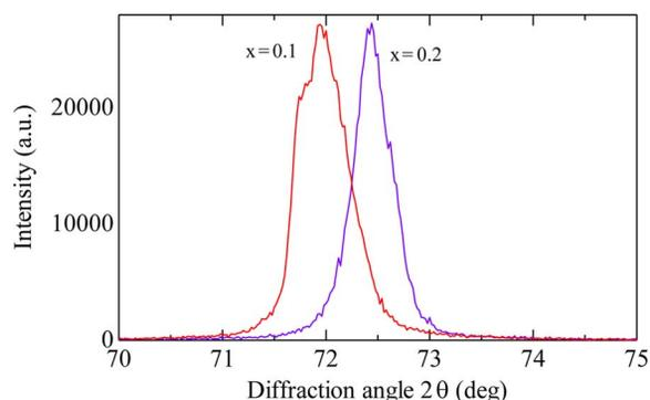
Fig. 3. The (422) diffraction peaks from the CZT layers grown with Zn-concentrations of 0.1 and 0.2 in the precursor. The Zn-concentrations were varied by controlling the supply ratio of DMZn, keeping the total supply rate of group II sources constant.
