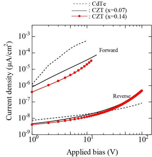
Fig. 5. Typical room-temperature  $I - V$  characteristics of the CZT diodes fabricated with different Zn-concentrations ( $x = 0.07$  and  $0.14$ ). For comparison  $I - V$  characteristics of a CdTe diode is also presented.
