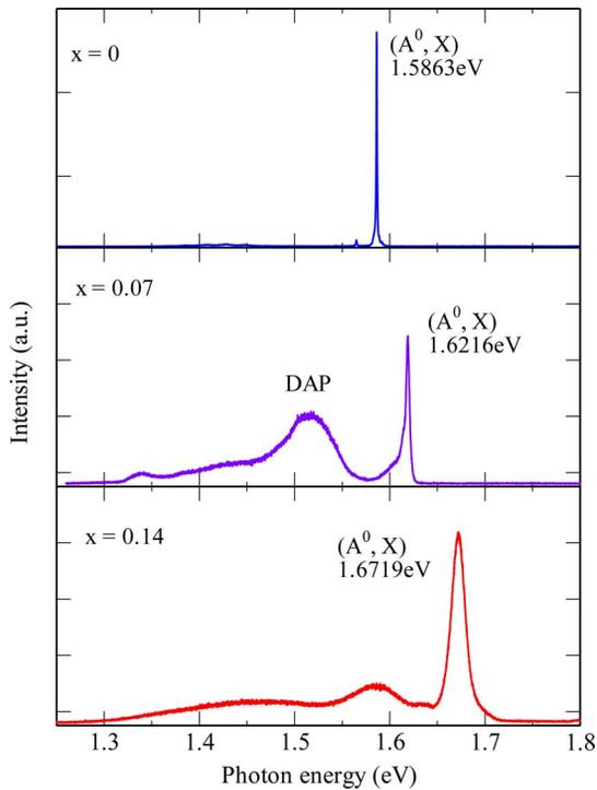
Fig. 4. The 4.2 K PL spectra of CZT layers with different Zn-concentrations of 0.07 and 0.14, and that of a CdTe ( $x = 0$ ) layer. Zn-concentration of the epilayers was determined from the XRD data.
