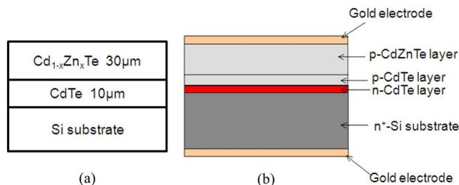
Fig. 1. (a) Sample structure used for CZT growth with different Zn-concentrations, (b) cross-sectional diagram of the CZT heterojunction diode fabricated. The CZT thickness was typically  $30 \mu\text{m}$  in (a), whereas it was increased to about  $80 \mu\text{m}$  in (b).
