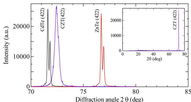
Fig. 2. Typical XRD patterns of CdTe, CZT, and ZnTe layers grown on (211) Si substrates. Zn-concentrations were varied as 0, 0.2 and 1.0 by controlling the supply ratio of DMZn, keeping the total supply rate of group II sources ( $\text{DMCd}+\text{DMZn}$ ) constant. The inset shows XRD  $2\theta$  scan of CZT layer in a wide range.
